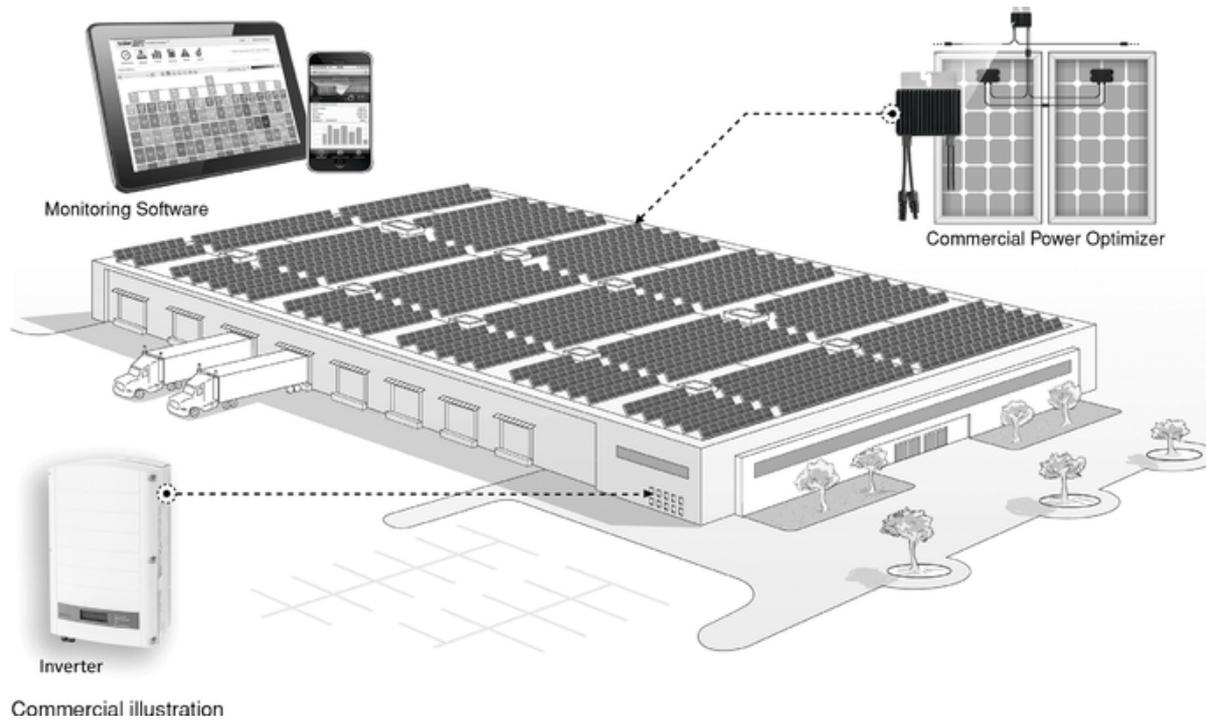
Our DC optimized inverter system maximizes power generation at the individual PV module level while lowering the cost of energy produced by the solar PV system and providing comprehensive and advanced safety features. Our solution consists of our power optimizers, inverters and cloud-based monitoring platform. Our solution addresses a broad range of solar market segments, from residential solar installations to commercial and small utility-scale solar installations.
