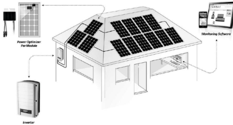
Our DC optimized inverter system maximizes power generation at the individual PV module level while lowering the cost of energy produced by the solar PV system and providing comprehensive and advanced safety features. Our solution consists of our power optimizers, inverters and cloud-based monitoring platform. Our solution addresses a broad range of solar market segments, from residential solar installations to commercial and small utility-scale solar installations.
