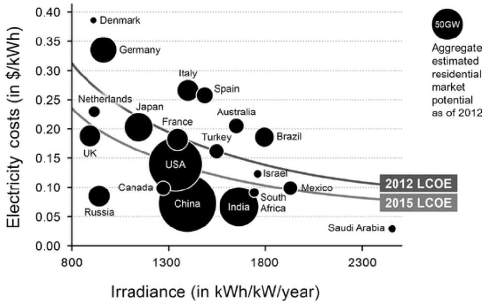
Note: LCOE based on 6% weighted average cost of capital, 0.7%/year module degradation, 1% capex as O&M annually. \$2.65/W capex assumed for 2012, \$2/W for 2015.
